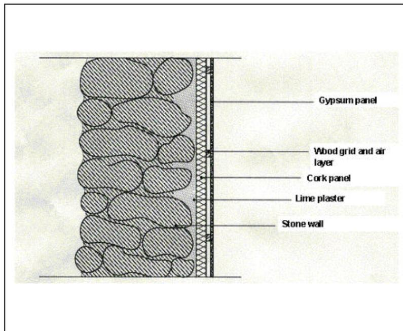
**Figure 1** – The starting solution proposed for external wall.
