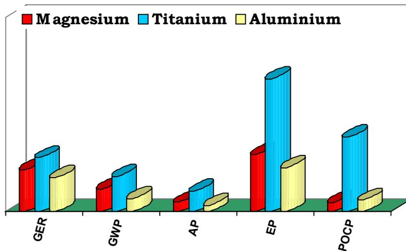
**Figure 2** - Main environmental results for Mg, Ti and Al
