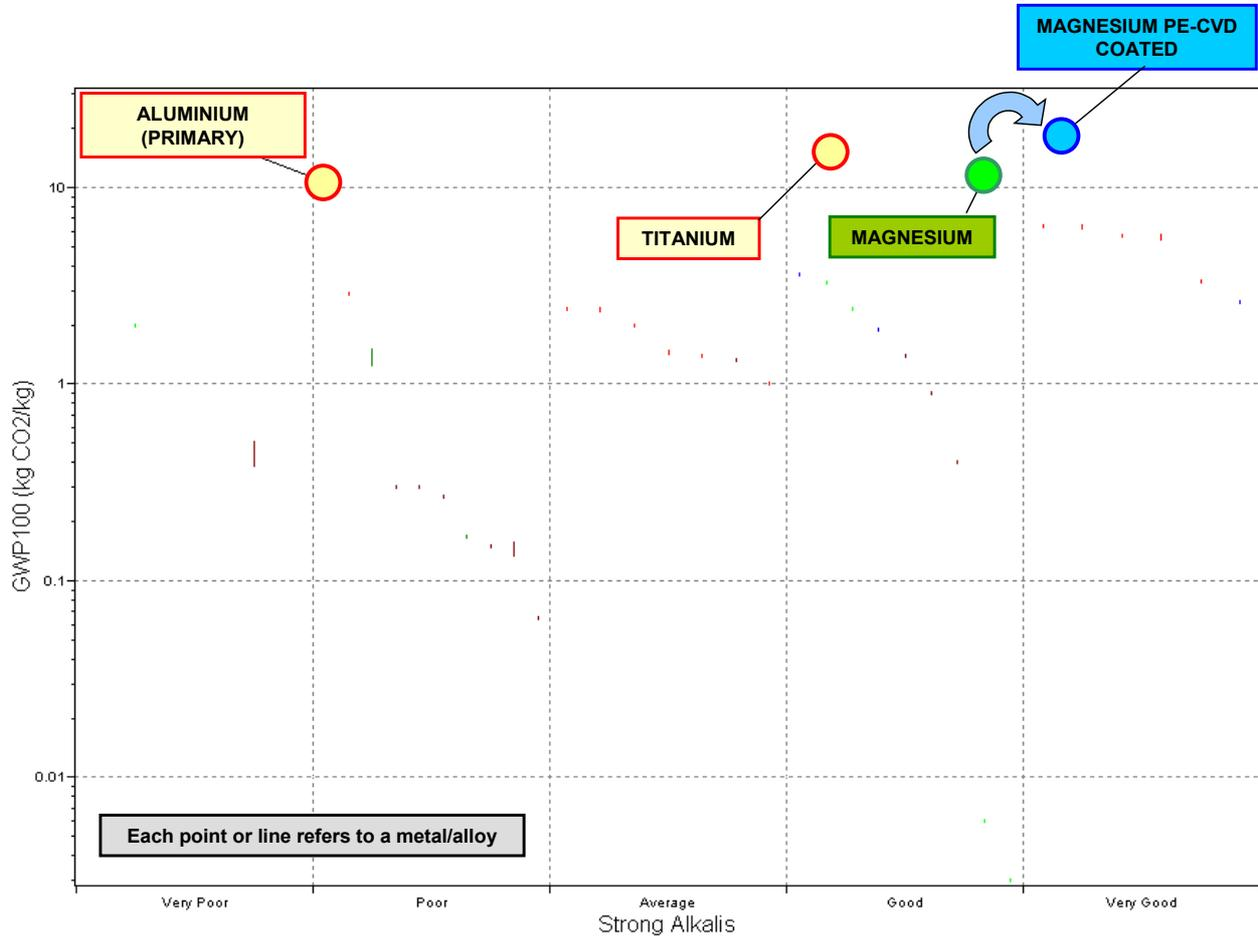
**Figure 4** – Eco-design applications: strong alkalis corrosion resistance vs GWP<sub>100</sub>
