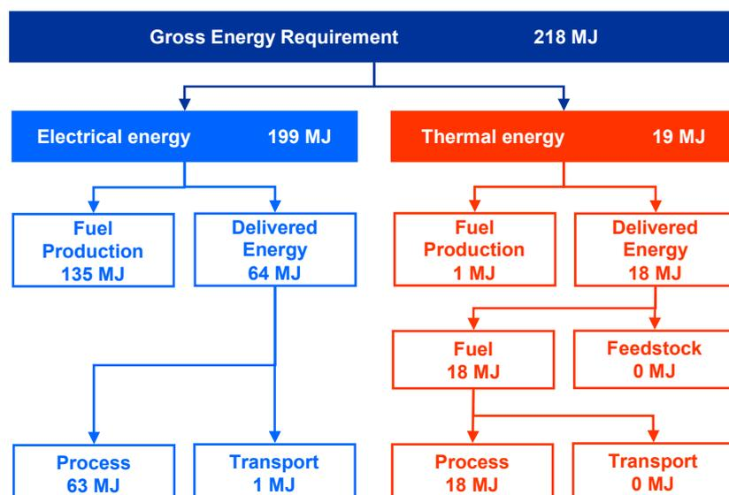
**Figure 2 – Gross energy results for magnesium production (data in MJ/f.u.)**
